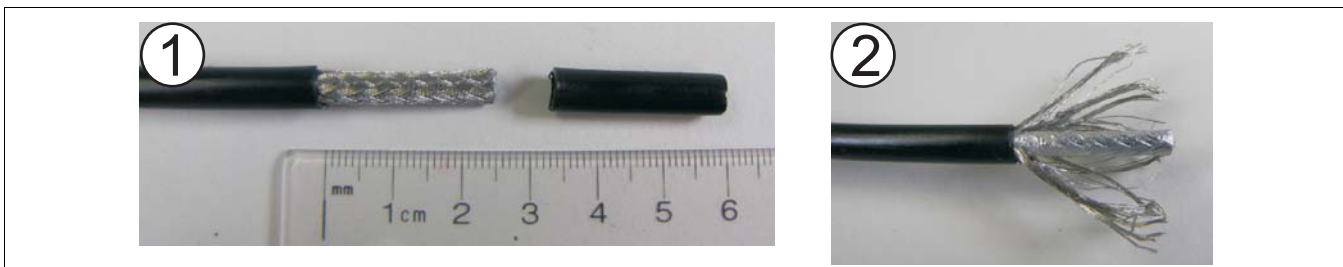
Figure 29: Preparing Mark 2 sensor cable step 1 & 2
