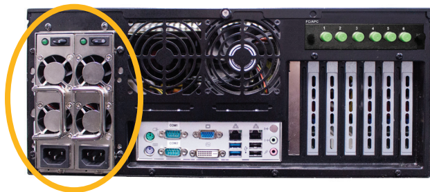
Two redundant, hot-swappable power supplies
